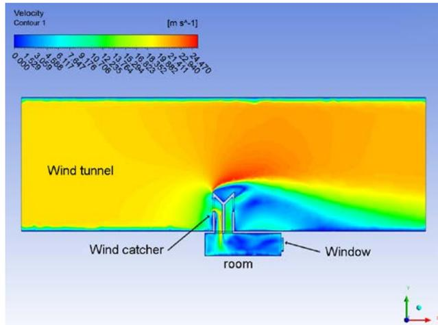
Figure 3. Velocity contours at 20 m/s.
