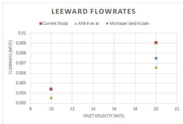
Figure 6. Comparisons between current study simulations and Afshin et al [2] and Montazeri and Azizan [25] for leeward flowrates.
