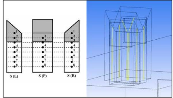
Figure 4. Montazeri and Azizan's model pressure taps [25] vs. simulation pressure line samples.
