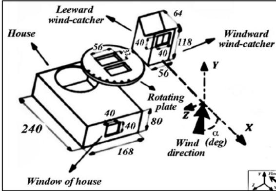
Figure 2. Afshin et al wind catcher model [2].
