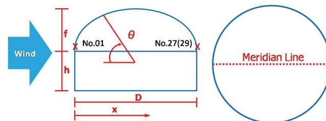
Figure 1. Geometric nomenclature and coordinate system
