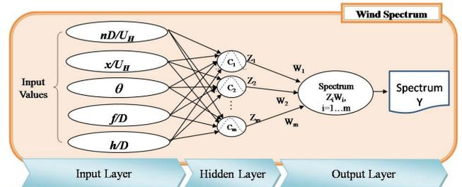
Figure 3. RBFNN Architecture for pressure spectra estimation of hemispherical dome roofs
