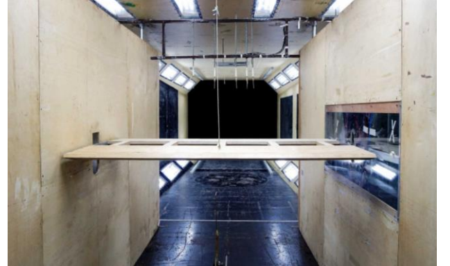
Figure 2 Wind tunnel pressure test setup
