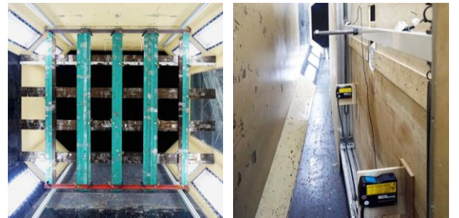
Figure 3 Turbulence simulation fence Figure 4 Springs and sensors
