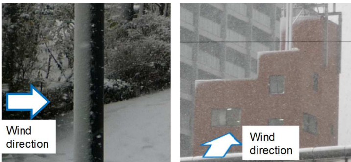
(1) Snow adhesion on concrete utility pole (2) Snow adhesion on building wall Figure 1. Examples of snow accretion observed outdoors.
