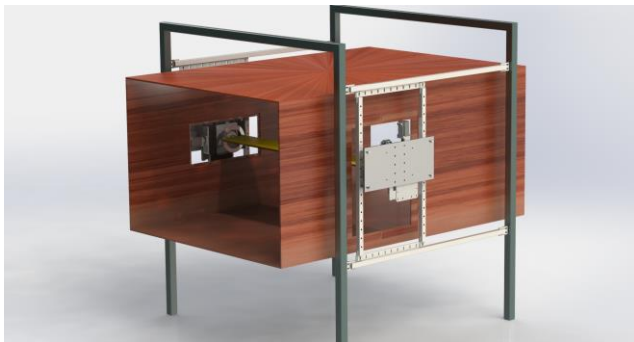
Figure 4. Experimental setup at NTNU [10]. Visualization of the part of the wind tunnel test section with the forced vibration rig.
