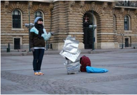
Fig.1: Picture of an automated bag sampler rig in front of the Hamburg town hall.
