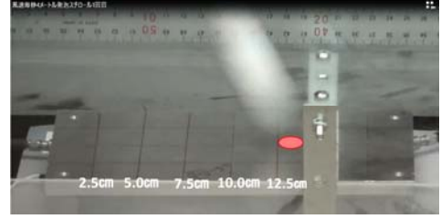
Figure 9. A photo of the falling sphere released in the wind speed U = 4 m/s. The sphere is going to hit the aluminium plate. The red circle indicates the hitting point observed from the video and its location x_h = 12.5 cm in this case.
