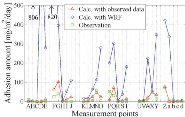
Figure 9. The amounts of salt on each member of the study bridge.
