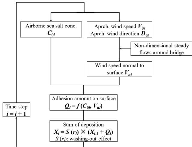
Figure 4. Calculation algorithm for sea salt amounts adhering on surfaces.
