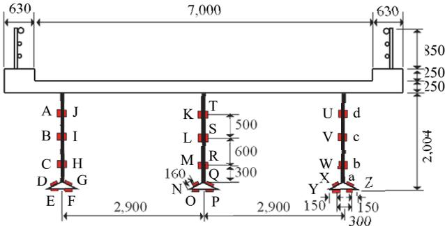
Figure 3. Cross-section of the study bridge and measurement points for salt amounts (A–d).
