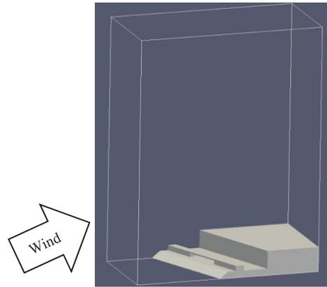
Figure 8. Computational domain for calculating a steady flow around the study bridge in the case of approaching wind angle relative to the perpendicular line of the bridge axis being 22.5°.
