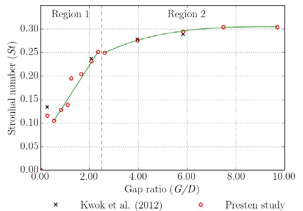
Figure 6: Strouhal number ( $S_t$ ) for different gap ratios.
