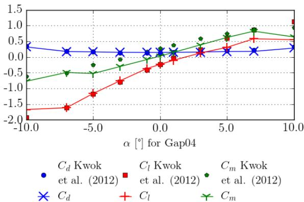
Figure 4: Force coefficients for Gap 04.
