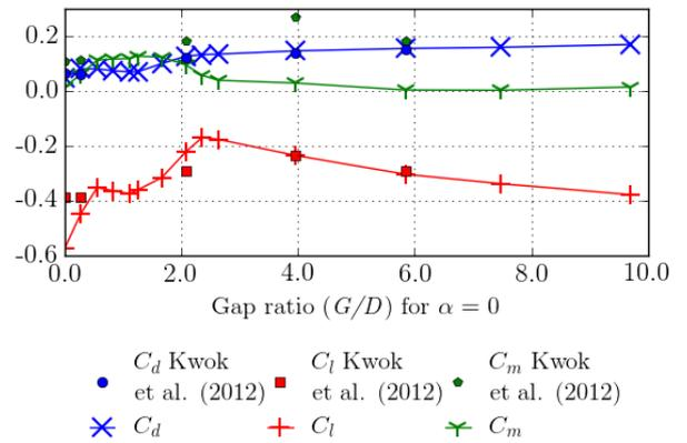
Figure 5: Force coefficients for different gap ratios at  $\alpha = 0..$
