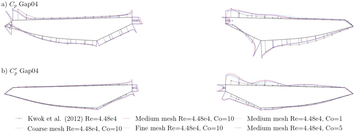
Figure 3: Mean pressure coefficient distribution and its standard deviation distribution. Negative values points outward the section and the height of the section is equal to a value of unity.
