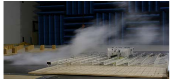
Figure 10 Wind tunnel model with smoke visualisation
