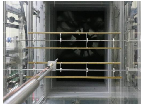
Figure 1. Closely spaced dual Darrieus rotors in wind tunnel.
