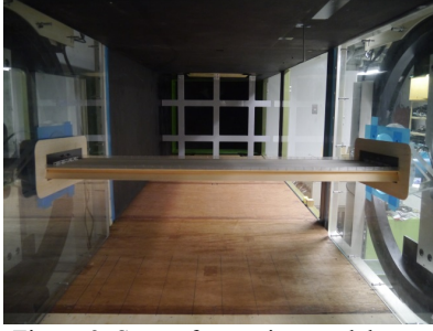
Figure 3. Set up for section model tests
