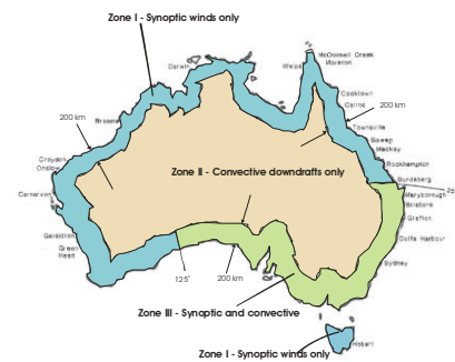
Figure 7. Zones in Australia showing dominant wind types for ultimate limits states (from [22])
