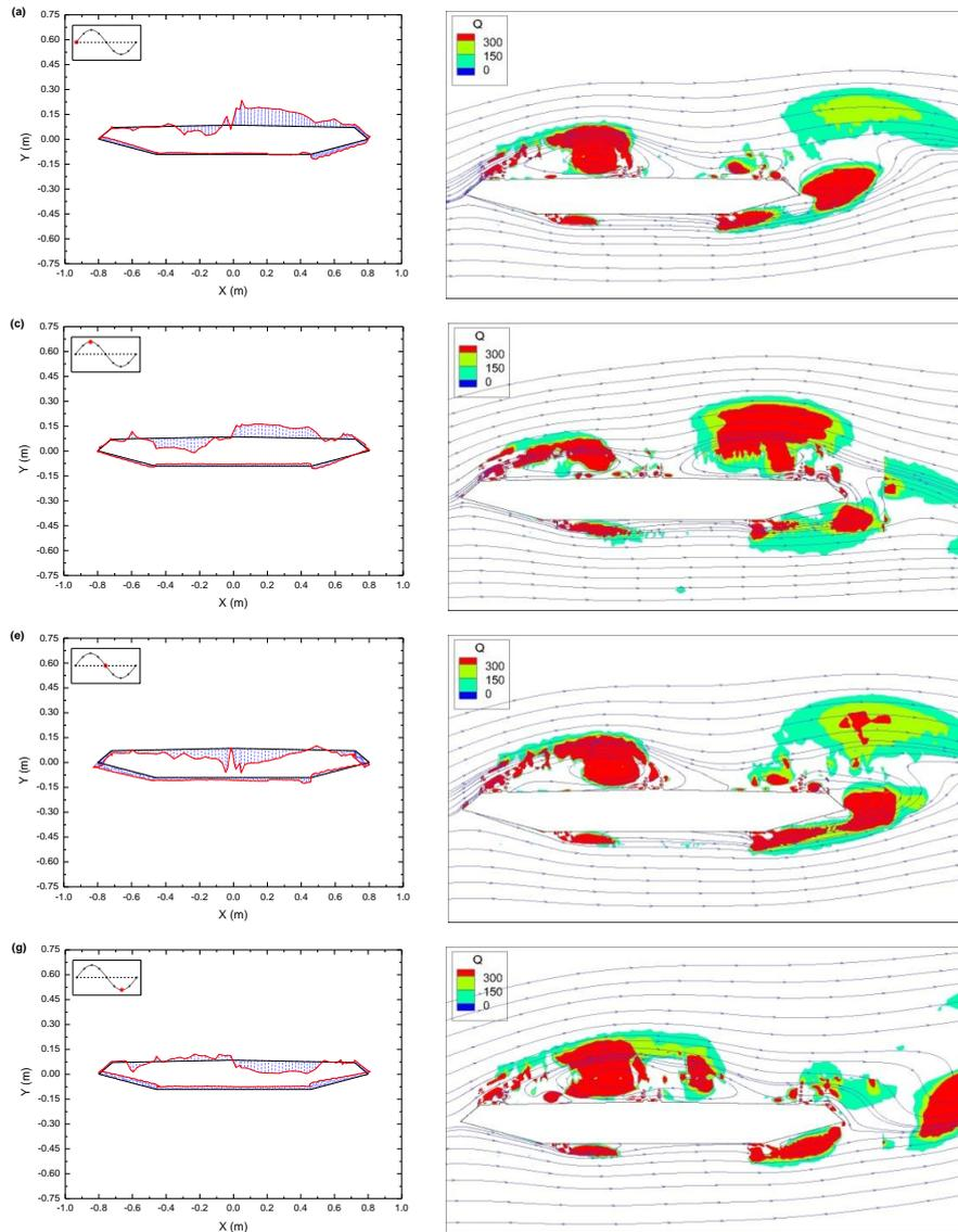
Figure 1. Distributed VIPs and vortex structures during one cycle of stable stage of VIV
