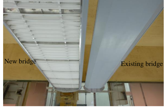
Figure 4. Section bridge model for the new bridge located upstream and the existing bridge located downstream for aerodynamic test under smooth wind
