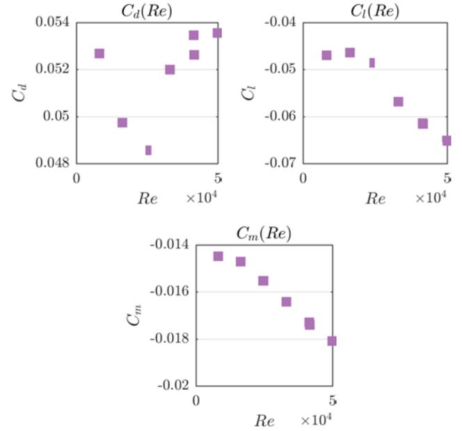
Figure 5. The scatter represents the lift coefficients obtained from the mean of the measured lift forces per unit length at zero degrees angle of attack ( $\alpha = 0^\circ$  deg) for different Reynolds numbers
