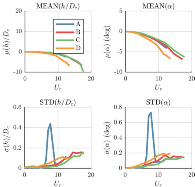
Figure 9. The mean vertical response relative to the depth of the central box girder,  $\mu(h)/D_c$ , are shown in the upper left plot. The mean rotations,  $\mu(\alpha)$ , are shown in the upper right plots. The lower plots shows the standard deviation of the vertical and torsional response. The legends in the upper left plot applies to all plots
