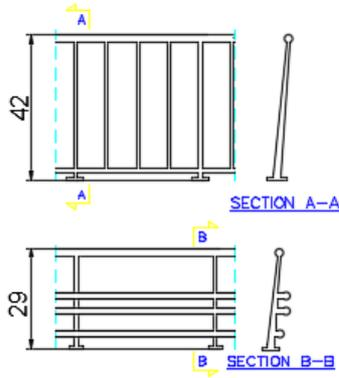
Figure 4. Railings used for the external decks (above) and the central deck (below). Dimensions are in mm
