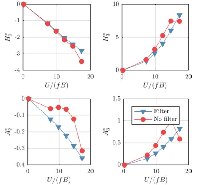
Figure 8. Aerodynamic derivatives estimated after digital linear phase bandpass filtering (triangles) and without digital filtering (circles)
