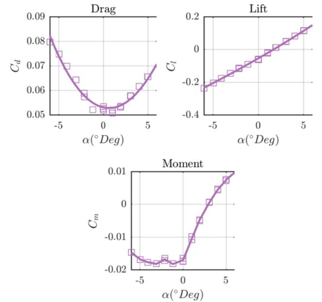
Figure 6. Static drag, lift and moment coefficients for the section model tested. Reynolds numbers effects might have caused small differences in the estimated coefficients indicated by the scattered values at the same angle of attack,  $\alpha$
