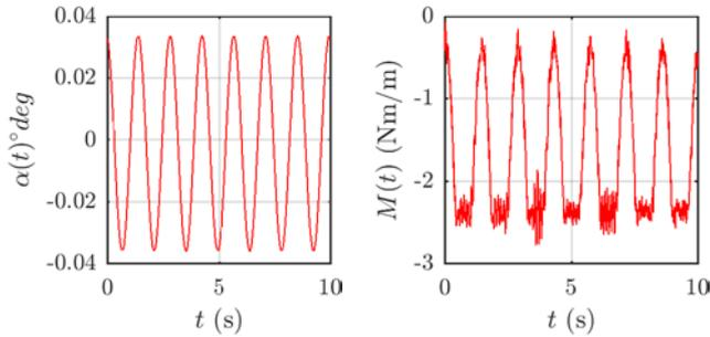
Figure 7. Time histories for the pitching motion (left) and measured moment (right) at  $U = 14.58$  m/s
