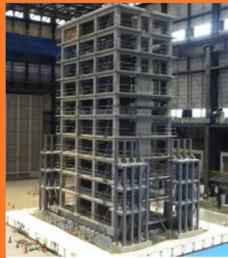
Figure 1: (a) 10-story RC moment frame building tested at the E-Defense shake table facility in Japan (Sato et al., 2017) and (b) Equivalent Demands for a structure location in Wellington, NZ
