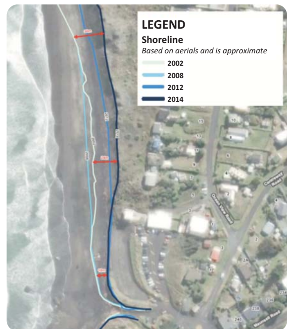
Map showing changes in the shoreline at Okariha, Port Waikato. Photo: GHD.
