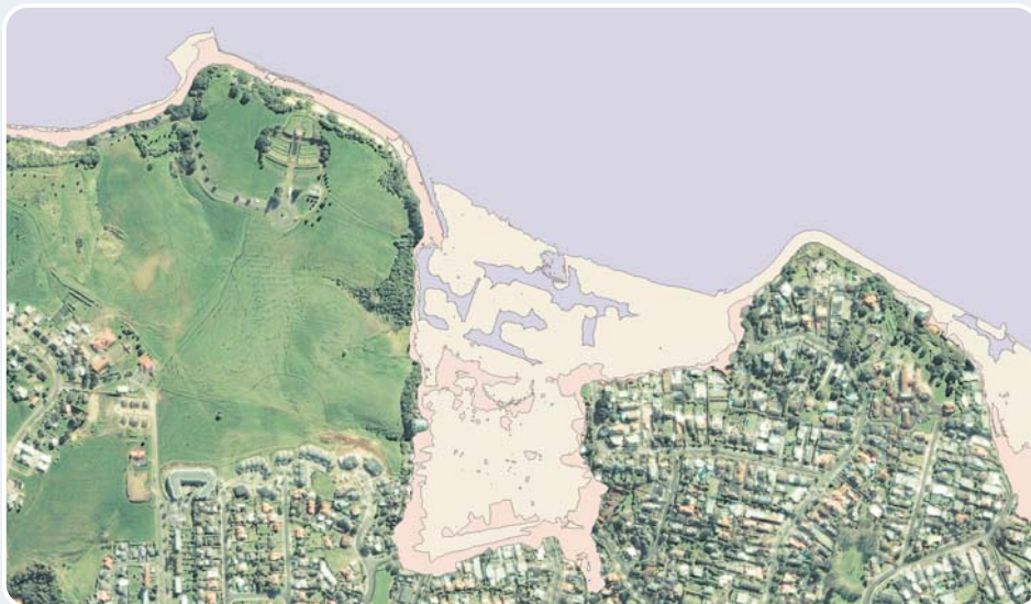
Top: Aerial photograph of Mission Bay. Centre: Mission Bay with present-day 1 per cent annual exceedance probability storm-tide plus wave set-up elevation superimposed (purple shading). Bottom: Mission Bay with present-day 1 per cent annual exceedance probability storm-tide plus wave set-up elevation superimposed (purple shading), plus 1-metre sea-level rise (light shading), and plus 2-metre sea-level rise (orange shading). Photos: NIWA.
