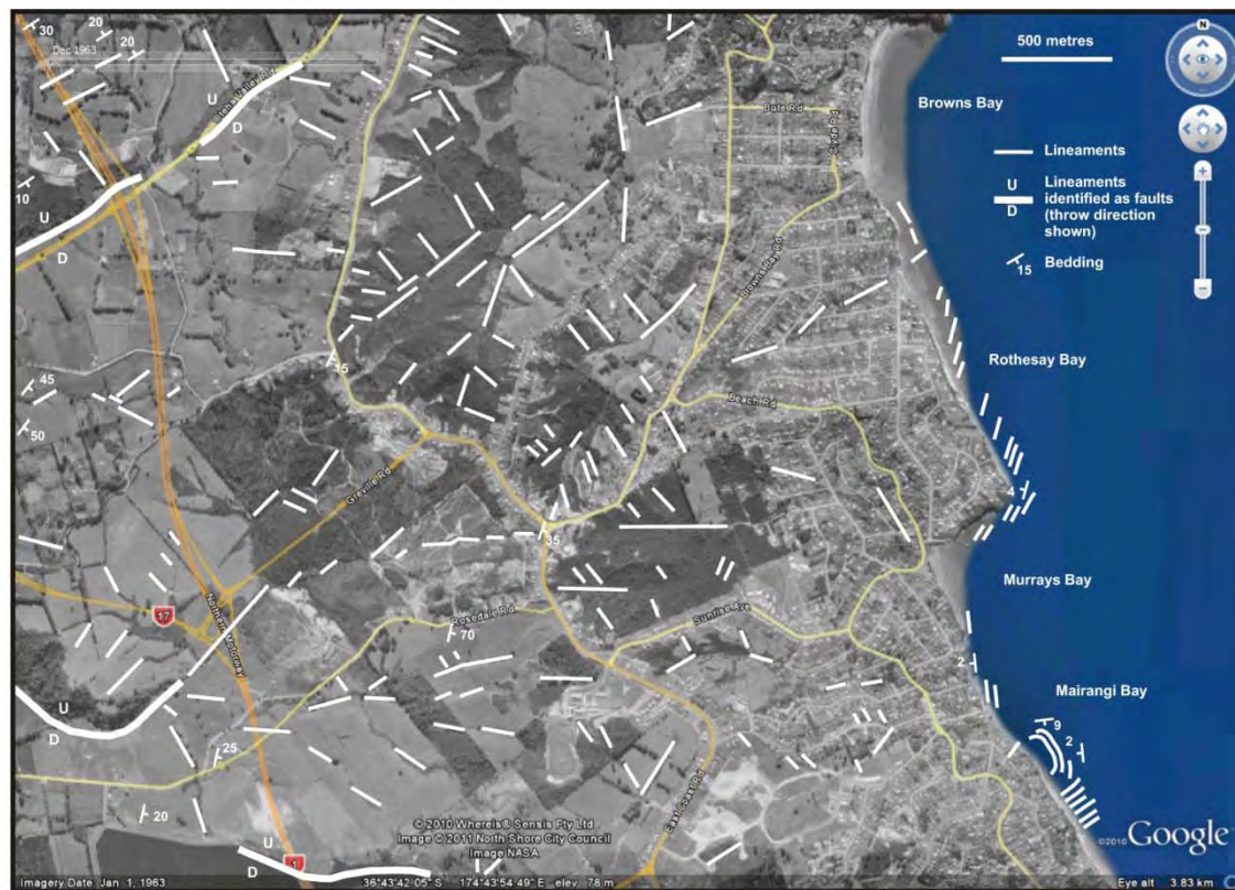
Figure 9: As in Figure 8, but with lineaments also superimposed on the historical Google Earth image. This is an example of how lineaments were mapped for the whole of Auckland, using 1960s stereoscopic aerial photographs. Bedding and lineaments identified as faults are also shown.
